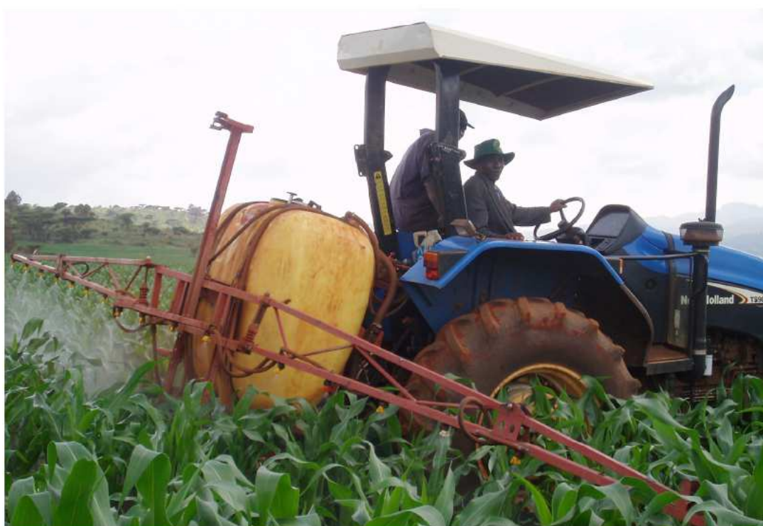
Plate 4.1b: Tractor mounted sprayer applying Bulldock suspension on young maize plants in Suam
