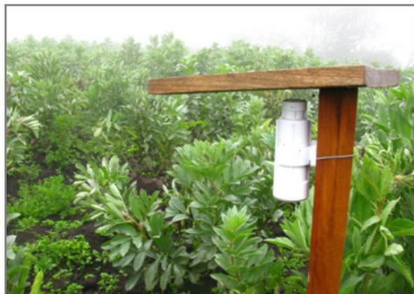
**Plate 7.** Temperature/humidity data-logger located next to a potato field in the Ecuadorian Andes.
