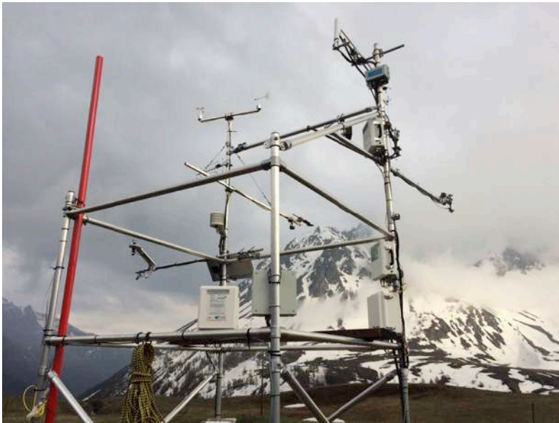
Figure 2. The flux tower at the Lautaret Alpine Station (SAJF) measuring energy and material flows in the soil-snow-vegetation-atmosphere continuum, © D. Joly.
